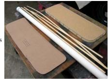
After soaking in hot water they could be carefully individually bent, without breaking, to the form shape. I used a length of 1 1/2" PVC pipe with an end cap, held vertically, and filled with hot water and a little ammonia, to soak the wood strips in. A small piece of cloth and a rubber band was needed to cover the top of the pipe to keep the wood strips submerged for the approximate hour they had to soak.
