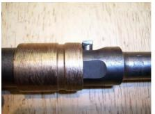
After the new end caps are installed and flattened you will re-stake the new caps.
