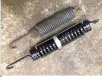
Now you have the challenge of removing your trough from the spring. This can be dangerous, so be cautious. The way we removed it was to use a floor jack and hook one end of the spring on the axle and the other over the top plate that would normally contact the car. As you pump up the jack, it extends the spring slightly so the trough can be removed after you remove the hose clamp. Lowering the jack releases the old spring. The process can now be reversed with the new spring.
