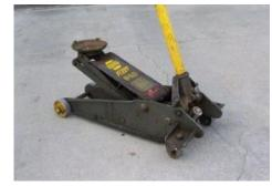
all. If filling with fluid and purging air from the system do not restore function, there is probably internal leakage, even though fluid is not leaking from the jack. From what I have read, forty years of service is a reasonable time for a hydraulic jack to operate before it needs a rebuild.
