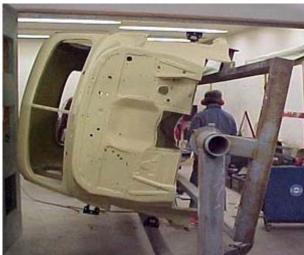
The only non stock part is the motor. I used a 1959 Chev 6 cylinder. I like high tech options like oil pumps, insert bearings! I had the water pump modified to measure the same size as the original and a kit that made the valve and side covers look like 1948.
