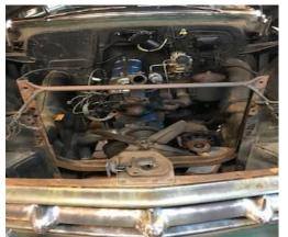
I now lifted the radiator support frame with the top wiring harness as an assembly, about 4", and braced it it with a short 2x4 piece of wood. (No need to do all of the other steps as shown in the book, unless my '53 design is different from the earlier models). At this point, I could reach the Harmonic Balancer head on.
