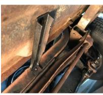
Next, I removed 2 bolts holding the center bracket attached to the front fender skirt.
