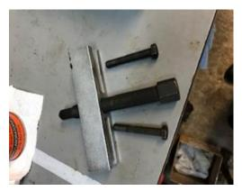
I drove to O'Reilly's Auto Parts and rented the Timing Gear Removal Tool kit (67010); actually, it's free as long as you return it within 48 hours.
