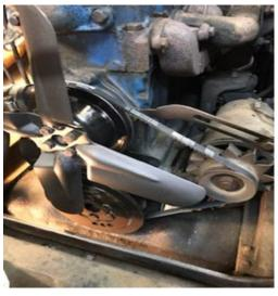
I bought a good used Harmonic Balancer from Old Car Parts in Portland, OR for \$75. I then shipped it off to Damoer Dudes in California. They rebuilt it for \$220. I also replaced the gasket and oil seal for the timing cover, fan belt, and the top radiator hose. Total cost with shipping was just over \$400.
