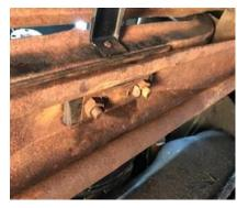
So I chose to approach things differently and removed all of the bolts securing the radiator support frame: to do this, I had to remove the battery and tray to reach the bolts on the passenger side. I then removed the 2 bolts and 4" flat bar with rubber on the underside of the support frame.
