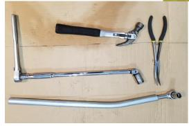
needle-nosed plier with a curved tip; a combination crescent wrench and vise grip tool; and a flexible screwdriver for adjusting breaker points through the sliding window on the distributor.
