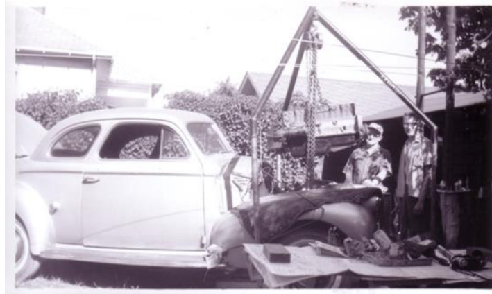
Installing the overhauled 216 Engine at 97,512 miles. My Dad and brother helping, June 1967
