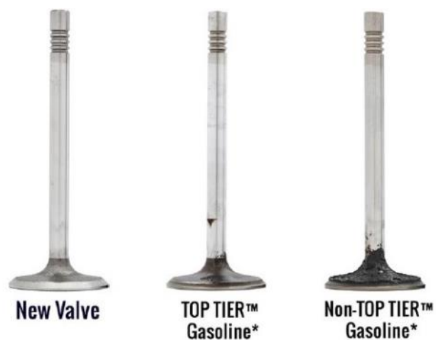
Intake valve comparison showing a new valve compared to the results from the 100-hour engine test. PHOTO: AAA
