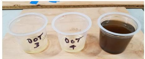
Another bad feature of this fluid pollution is that as the water content increases, the boiling point of the brake fluid lowers (fairly dramatically). This will cause a noticeable brake-fade from excessive braking which is experienced during heavy use of your brakes down a large downhill grade, during emergency stops, or "spirited driving".
